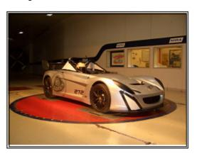
We also took the opportunity to optimise the location and angle of incidence for both the standard and optional wings and the front splitters, giving us an excellent downforce balance for the non-adjustable standard setup and a useful range of complementary settings for the optional adjustable wings.
